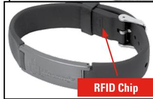
**NOTE:** *The RFID chip is located in the bulge of the wristband near the clasp. It is designed to be worn on the bottom of the wrist for maximum read distance.*
