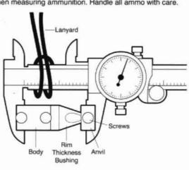
described in Safety Warning above, attach the anvil (short flat-top with slot) to the traveling blade of your caliper using the brass thumb screw inserted into the thick leg of the anvil. Attach the body (tall red with hole) to the stationary blade of your caliper with a brass thumb screw inserted into the thick leg of the body. Close the blades of the caliper and align the anvil with the body ensuring that they are flush and straight with each mating surface. Tighten brass screws.
