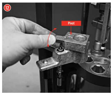
3 For small rifle cases, place the Pivot Adapter Bushing into the hole of the Pivot Adapter.
