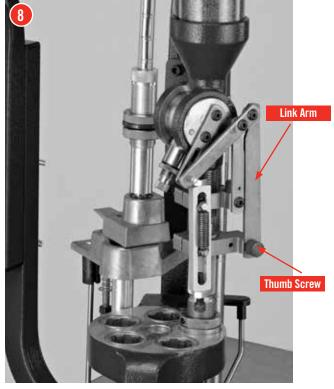
Attach PTX Powder Measure Stop. Attach Spring (14). (For adjustment, refer to Chart on page 43).
