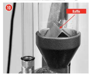
Drop Baffle into Powder Hopper to prevent powder bridging and help produce consistent charges.
