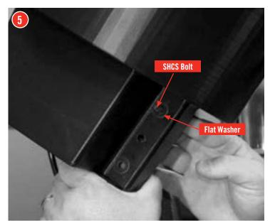
6 Place a ¼-20 X 2 SHCS Bolt (30) with one ¼" Flat Washer (31) through the bottom hole of the Bullet Feed Hopper and the Square Tubing Mounting Bracket.
