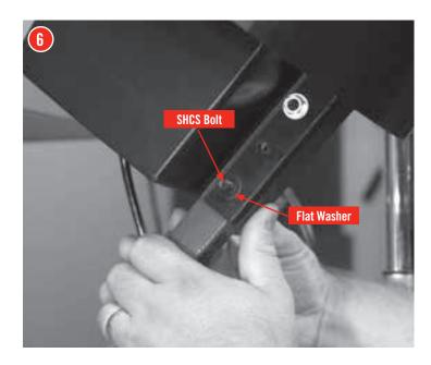
Place a ¼" Flat Washer (31) over the end of each of the two Bolts just previously place through the Bullet Feed Hopper and Square Tubing Mounting Bracket.
