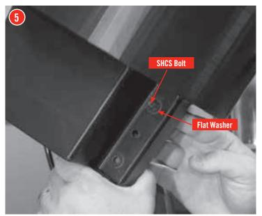
Place a ¼-20 X 2 SHCS Bolt (30) with one ¼" Flat Washer (31) through the bottom hole of the Bullet Feed Hopper and the Square Tubing Mounting Bracket.
