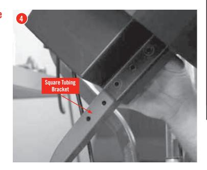
Place a ¼-20 X 2 SHCS Bolt (30) with one ¼" Flat Washer (31) through the top hole of the Bullet Feed Hopper and the Square Tubing Bracket.
