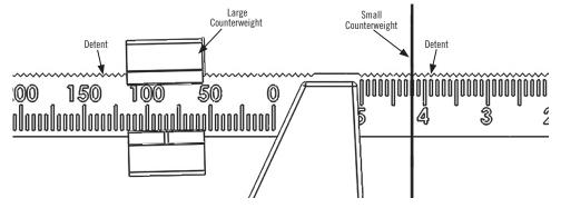
WARNING: The counterweights must be fully seated in the detent grooves to ensure accurate results.
