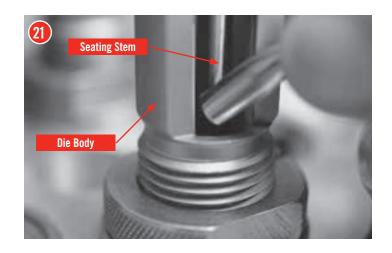
Set the bullet seat depth by lowering the press ram, threading the Seat Adjust Screw (42) into the die and raising the press ram again until the desired seating depth/cartridge length is obtained. Make sure the Crimp Adjust Screw (46) does not move when adjusting the seating depth.
